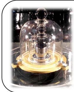
Some of the units used to have reference to physical artefacts, the most famous being the International Prototype of the Kilogram (IPK), which was held in a vault in Paris. The problem with using a physical artefact to define the unit, is that it is subject to changes in properties over time. Since the creation of the IPK in 1889 variations in environmental conditions caused the mass to change, so the definition of the kilogram was linked to something that was unstable over long periods of time.
